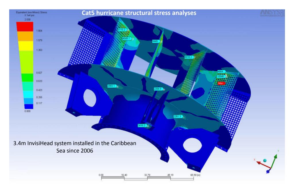
Equivalent (Von-Mises) Stress modeling for Cat5 hurricane of a 3.4m InvisiHead system installed in the Caribbean Sea in 2006; the IH system has been in operation ever since, delivering the design capacity under all weather conditions. The system it replaced was infested by zebra mussels and was rendered useless and had to be replaced
