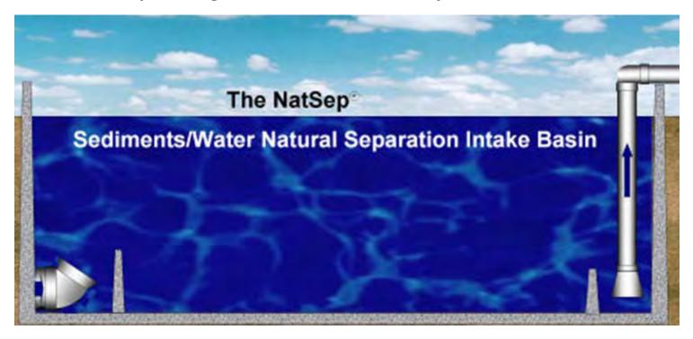
The NatSep is designed to separate any sediment that may flow through into the basin as part of the water flowing into and through the IH. By the time the flow reaches the seawater pump bay it is free of sand and weeds. The NatSep design upgrading is included in the intake system performance improvement.
