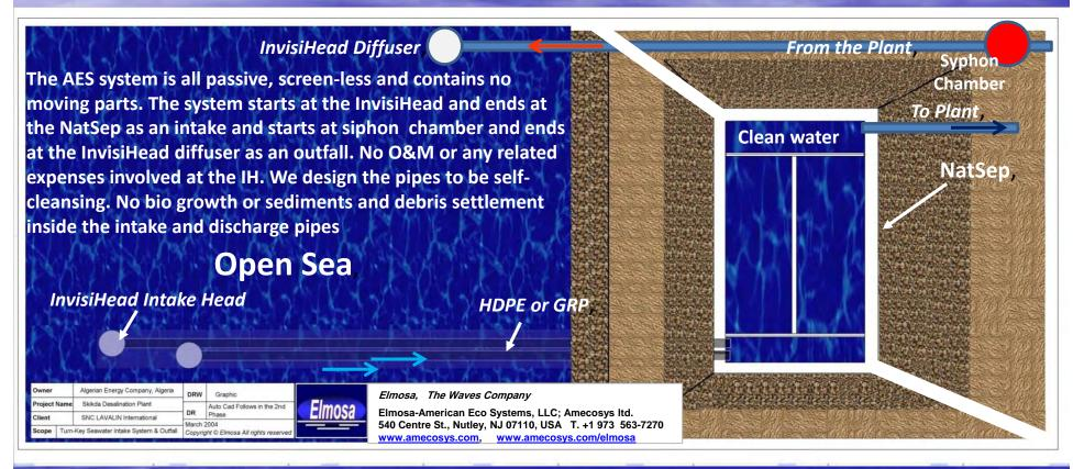
We at American Eco Systems design seawater intakes and outfalls to be maintenance – free, to provide full flow capacity under all operation and weather conditions non-stop for over 50 years. The system is environmental-friendly and supports biodiversity; the 4-compartment NatSep delivers clean water to the pumps; uninterrupted operation during the one-day cleanup every 5 years or so.
