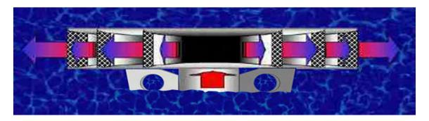
The IH discharges effluent in a 3-D round surround out flaring diffusing action. The effluent is in effect dispersed and diluted in an extremely large volume of the ambient water within a limited space surrounding the IH structure. The discharged effluents fade away into the ambient and reach equilibrium within a short time after diffusing.
